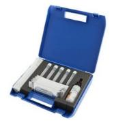
Swab Test Kit allows Legionella detection from surfaces and biofilms. Instead of collecting water, you swab the area to obtain biofilm sample. Since Legionella grows in biofilms the swab kit allows sampling directly from the source, which makes it very accurate and highly sensitive. This kit is very useful for locating the source of infection. The sensitivity of the kit is 200 CFU/swabbed area. The Swab Tests can be purchased in sets of 5 or 1. (€64.94/for one or 5 for €318.50)
